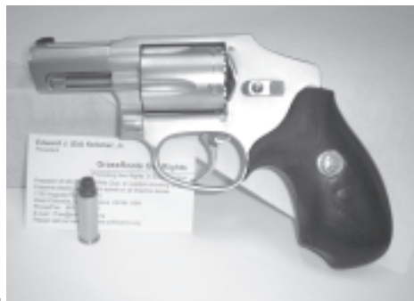
Revolver is S&W 442, nickel plated, .38 Special with a Wiggins custom barrel.
