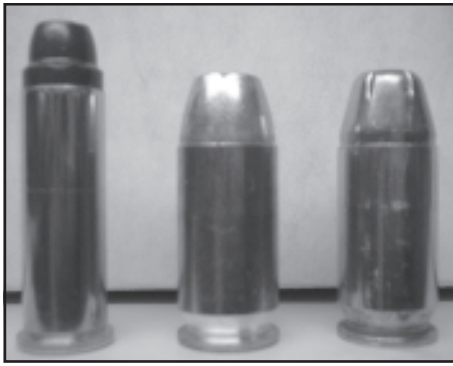
The .38 Special on the left is a Federal NyClad 158 grain lead hollow point. The .45ACP cartridge in the middle is a Speer 230 grain jacketed hollowpoint that did NOT feed properly in the Backup 45. On the right is a Hornady .45ACP +P 230 grain jacketed hollow point that fed and shot well in the Backup 45.
